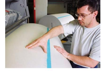
*UV-Cured* Acrylics and rubber. The reactive systems process achieves fluidisation through liquid components and solidification by curing (radiation-initiated reactions). Strong points: thin to very high thickness, high cohesion, good reversibility.
