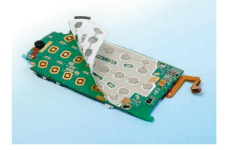
**Electronic** A wide range of PSAs is used for special applications in the manufacturing and assembly of electronic components. Tapes are used for the bandoliering of electronic components, masking connectors on printed circuit boards and many other applications.
