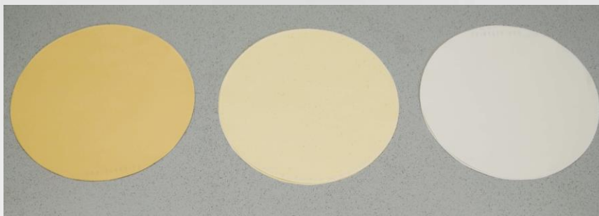
Figure 1: Colour of release liner. Left: dark glassine release liner; right: light glassine release liner; centre: glassine release liner resulting from recycling dark and light release liners together. Photo courtesy of UPM Specialty Papers.
