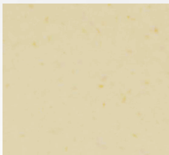
Figure 2: Impact of release liner colour on recycling outcome. Detail of recycled glassine release liner resulting from mixing dark and light release liners; note the dark specks on the surface. Photo courtesy of UPM Specialty Papers.
